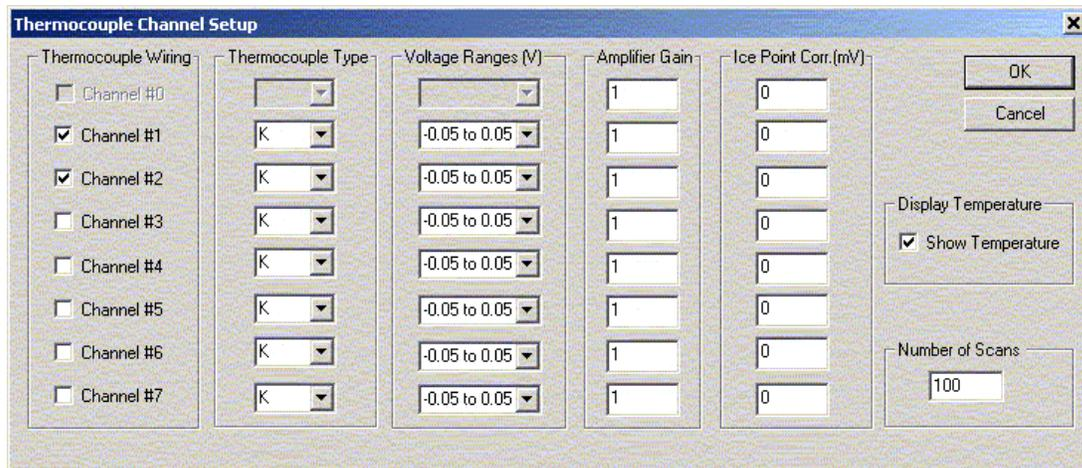
After the user clicks “Display” in the thermocouple menu, a display box appears showing the voltage for all selected channels, as well as the corresponding temperature, if this option was selected in the thermocouple setup menu. The program scans channel #0 (the spectrometer), followed by each selected channel in sequence, then repeats this cycle for the number of specified scans.
