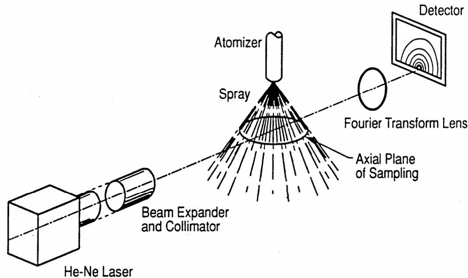
Diffraction signal analyzed to provide transient drop sizes
