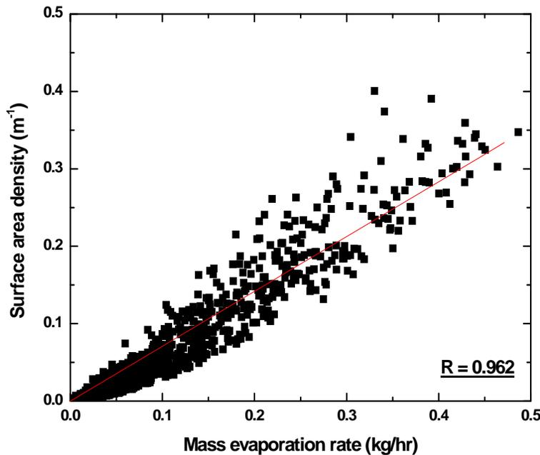
Correlation coefficient (R) of spray parameters with evaporation
