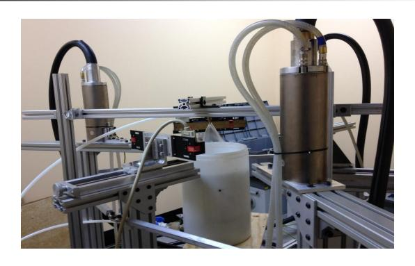
Three sources in fan beam configuration within a 12 ft x 12 ft x 6 ft lead lined chamber
