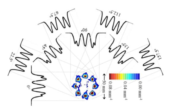
➤ Tomography of extinction data with a sampling frequency of 9.4 KHz
