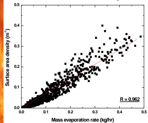
Drop size = 0.681Velocity = -0.239Mass flux = 0.903Surface area density = 0.962
