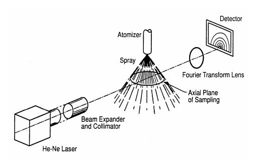
Diffraction signal analyzed to provide transient drop sizes
