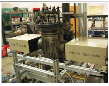
Pressure vessel fitted with AP400 patternator Maximum field of view is 100 mm
