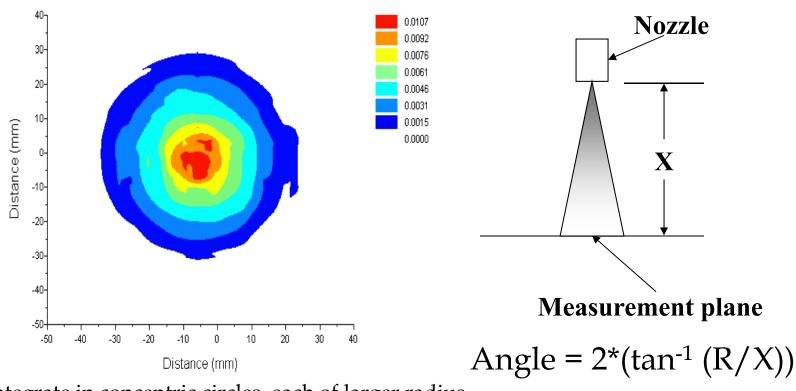
Integrate in concentric circles, each of larger radius, until 95% of Spray Surface Area Density is found.
