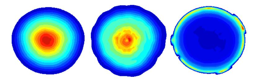
Mean, RMS, and RMS/Mean of drop surface areas to look at different aspects (uniformity, steadiness, drop size variations, presence of streaks and voids) of the spray
