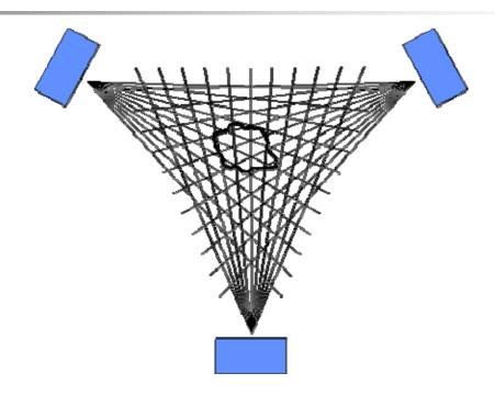
Emission tomography with high spatial resolution Used for non-homogeneous paths Detailed profile-not an online monitoring tool
