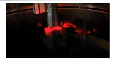
Liquid nitrogen with a flow rate of > 4 GPM Atomization quality is not very good Cloud of water vapor quickly forms in measurement zone Clear for about 1 minute Drop size/velocity too dense for optical patternator Flow rate does not stay constant
