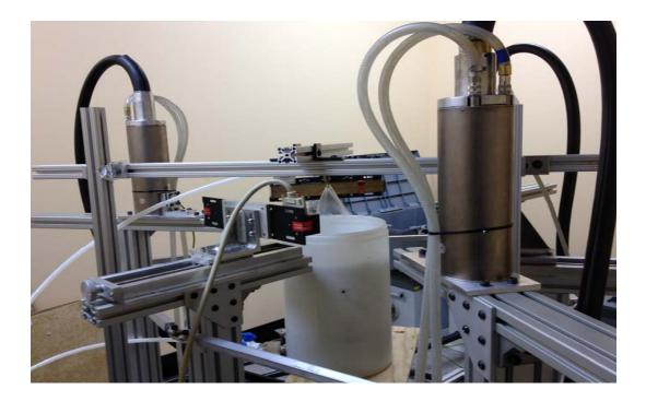
Three sources in fan beam configuration within a 12 ft x 12 ft x 6 ft lead lined chamber
