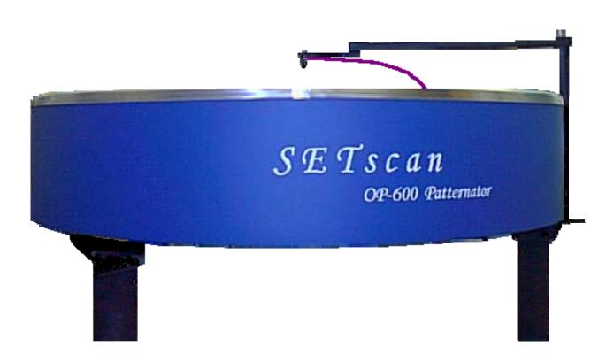
High frequency, optical patternator for sprays
