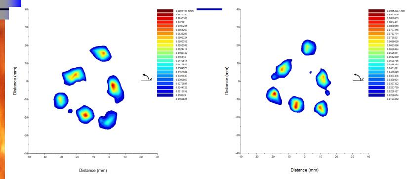
A has higher surface area density (implying smaller drops) Standard deviation and spread amongst plumes higher for A Higher mean plume angle and spread in plume angles for A
