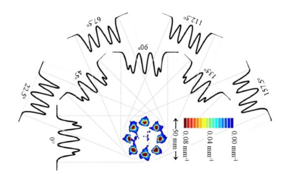
Tomography of extinction data with a sampling frequency of 10 KHz
